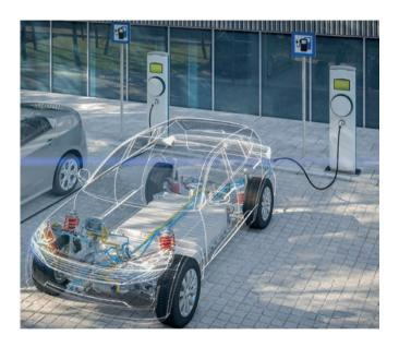
**Onboard charger:** This device takes the incoming AC electricity supplied from the charge port and converts it to DC power for charging the traction battery. It also communicates with the charging equipment and monitors battery characteristics such as voltage, current, temperature and the level of charge while charging the pack.
